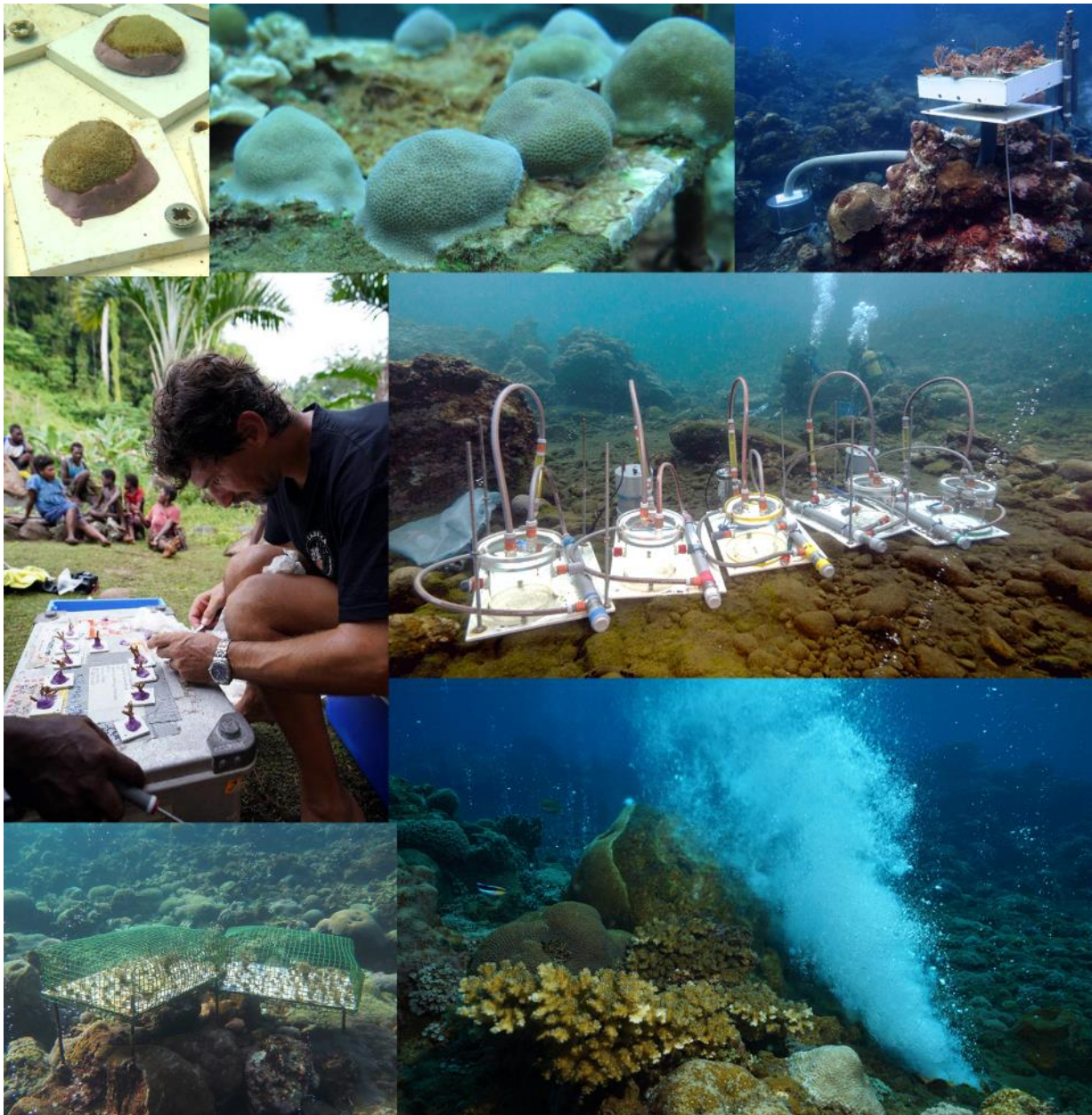
Fig. 4.8.2.2. Photomosaic showing the transplanted samples of Porites at the beginning and after 7 month at CO 2 seeps in Ambitle; the 'cathedral', i.e., the transplantation we did to study the combined effect of warming (note the tube trapping a hot emission) and OA on transplanted corals; some working on land with the special help from local people; the 6 respirometric chambers we used to measure the coral respiration; the second transplant setting and a nice vent eroding a Porites colony.
