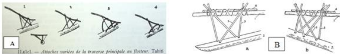
Figure 11. Attaches du balancier aux traverses. Sources Neyret (1974, A), Haddon et Hornell (1975, B).
