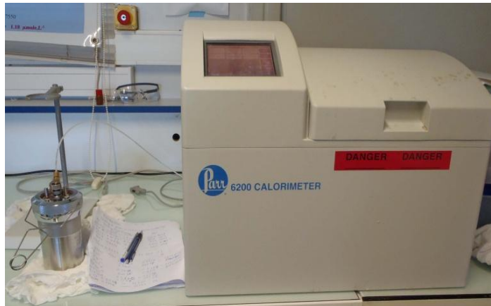
Figure 2.6. Calorimetric bomb used to determine energy content of samples.
