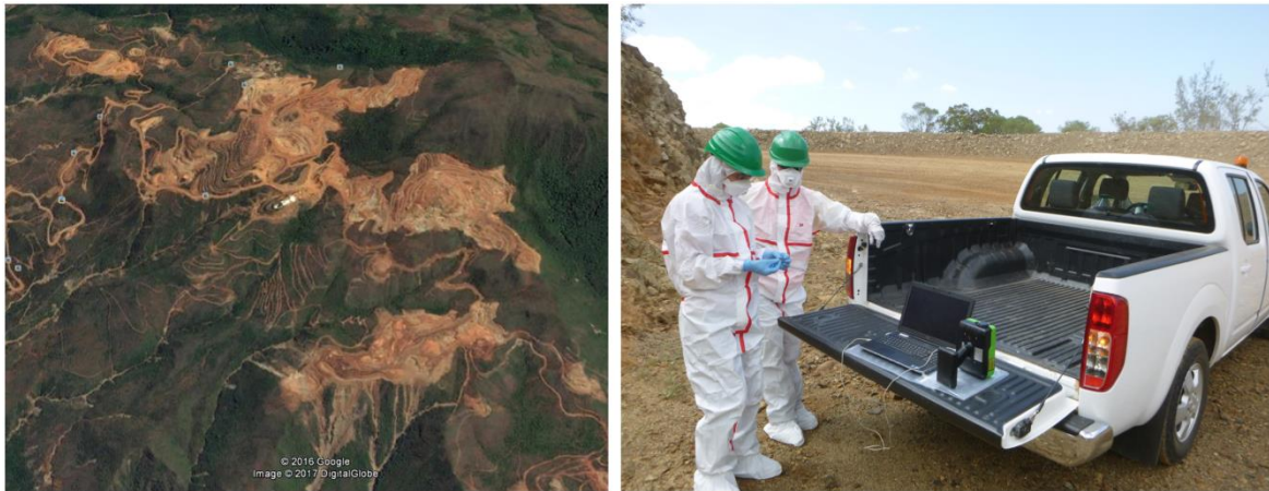
Figure V.2. Portable Raman test at the open mine of Tontouta (New Caledonia).
