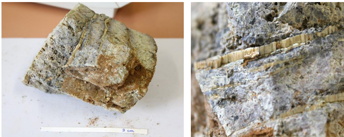
Figure II.23. Example of serpentinitized peridotite from serpentine sole horizon. Cross-veinlets a few millimetres wide of chrysotile are observed (Sample 53).
