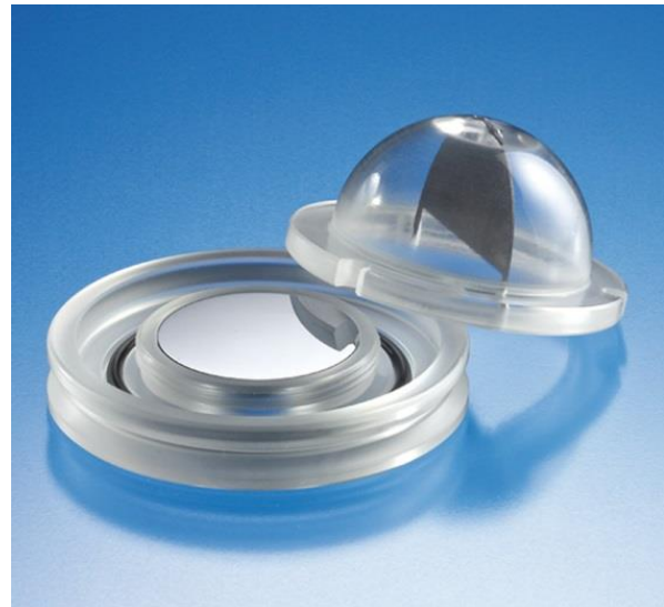
Figure II.17. Example of benchtop XRPD instrument equipped with dome-type zero-background sample holder (Bruker-AXS D8 Advance, available at SCVSA Department, University of Parma).
