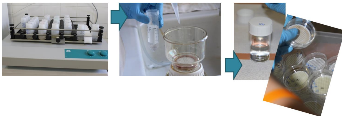
Figure IV.1. Batch leaching experiments: leaching on a shaking table, filtration, solution analysis and filter weighting.
