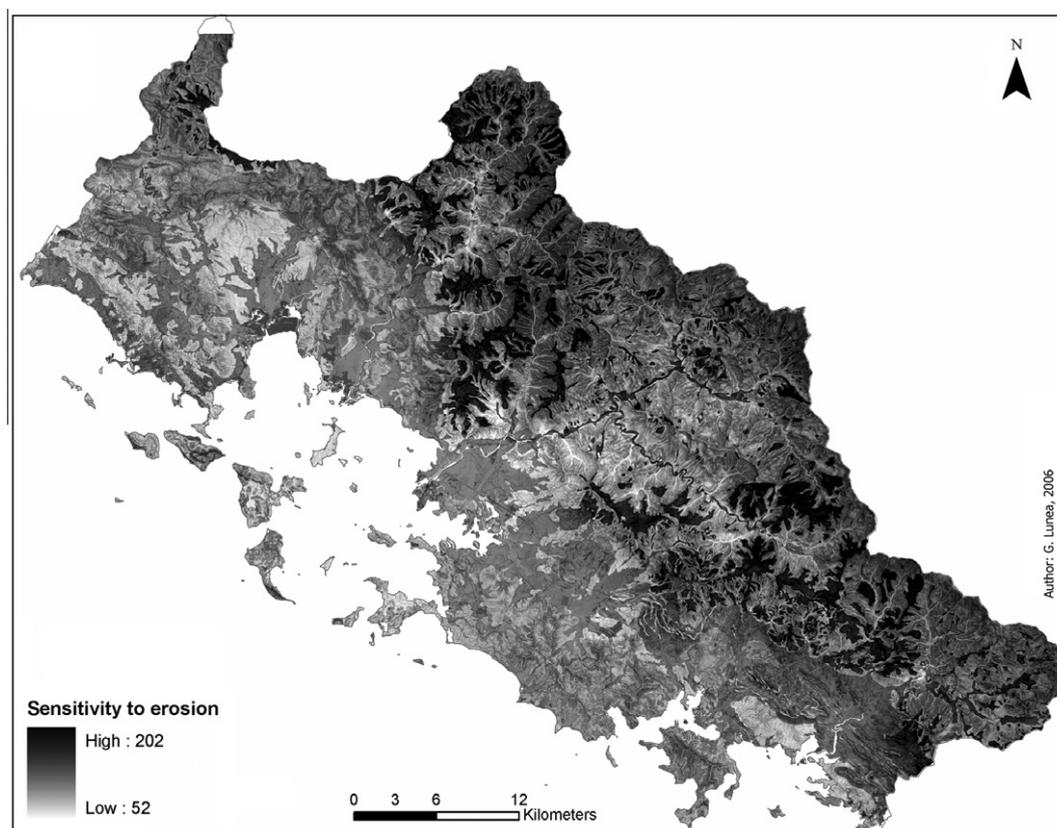
**Fig. 5.** Spatial distribution map of sensitivity to erosion by multi-criteria and weighted cross-referencing. This result highlights a high erosion hazard in denuded areas covered by laterite with steep slopes.
