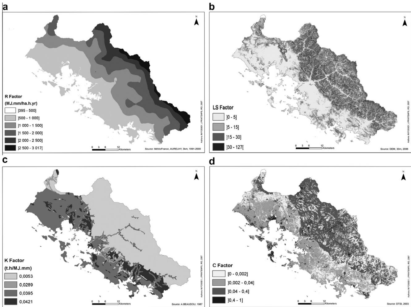
**Fig. 4.** Four factors are used for the application of Universal Soil Loss Equation: the rainfall and runoff factor (R), the length and slope steepness factor (LS), the soil erodibility factor (K) and the cover management factor (C).
